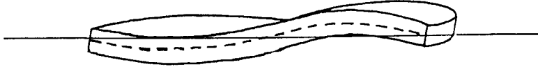
Fig. 13.1. A shell is ‘shallow’ if, in its reference configuration, the deviation of its middle surface from a plane is (up to an additive constant) of the order of the thickness of the shell
